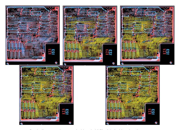
Gradually tracing the entire double-sided PCB whilst building the schematic.
